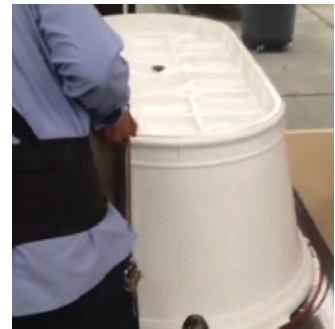
Mold being removed on tub made of Hydroluxe SS after it has become solid.
