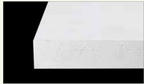
Surface coated mineral composite with void areas
